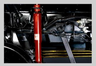
Shock Absorber (Rear) New hydraulic dampers improve handling and ride qualities for a more precise and comfortable travel.
