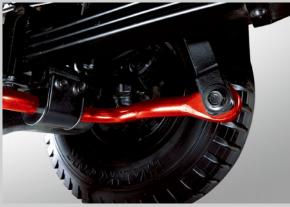
**Stabilizer Bar (Front / Rear)** Stabilizer bar increases structural rigidity to more effectively absorb vibration and road shocks.
