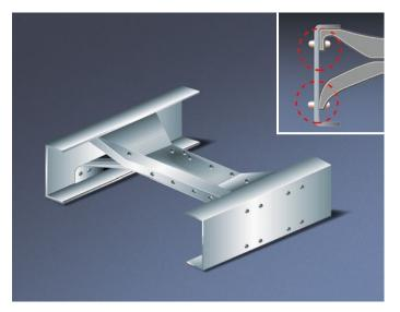
**Cross-member Reinforcement** To resist torsion and flexing and achieve the highest possible degree of rigidity and strength, heavy duty cross-members are added.
