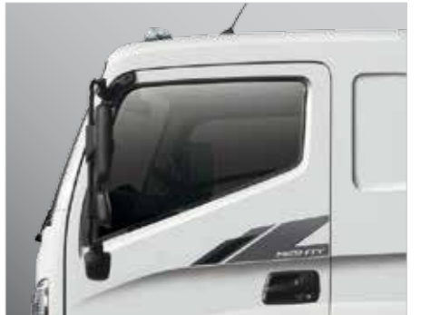
Taller, Wider Side Glass A taller, wider side window provides the driver with a much better view for safer driving.
