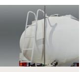
**Rear ladder** Water tank lorry HD65 ~ HD310 \* HD72/78/120 Ladder is attached to the side of tank
