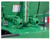
2-way valve (2 ea) Vacuum tank lorry HD65 ~ HD310 \* Suction or discharge under 3way valve set up \* Blow HD120 2.5'' Above HD170 3''
