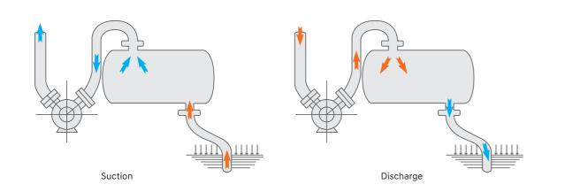
Air inside the tank is forced out by the vacuum pump which creates a pressure differential between the tank interior and exterior thus creating suction to collect waste. For discharge, the flow is reversed: Outside air is pumped into the reservoir which in turn forces the inner waste to be discharged.
