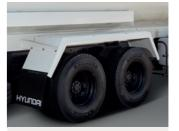
Fender Water tank lorry HD65 ~ HD310 \* HD65 ~ HD170 : Plastic HD260 - HD310 : Steel
