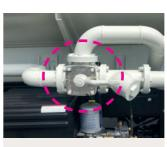
Pump (gear) Fuel tank lorry HD72 ~ HD260 \* Adjust amount of suction or discharge 4-way valve controller Fuel tank lorry HD72 ~ HD260 \* Set up between suction / discharge / stop / gravity
