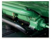
**4-way valve controller** Vacuum tank lorry HD65 ~ HD310 \* Suction / Discharge / Neutral
